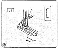
(3) The machine will automatically bartack and sew up the left side of the buttonhole.
